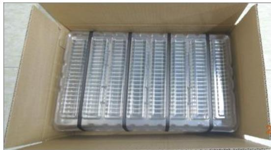
6. Seal the inner box by AzureWave tape
